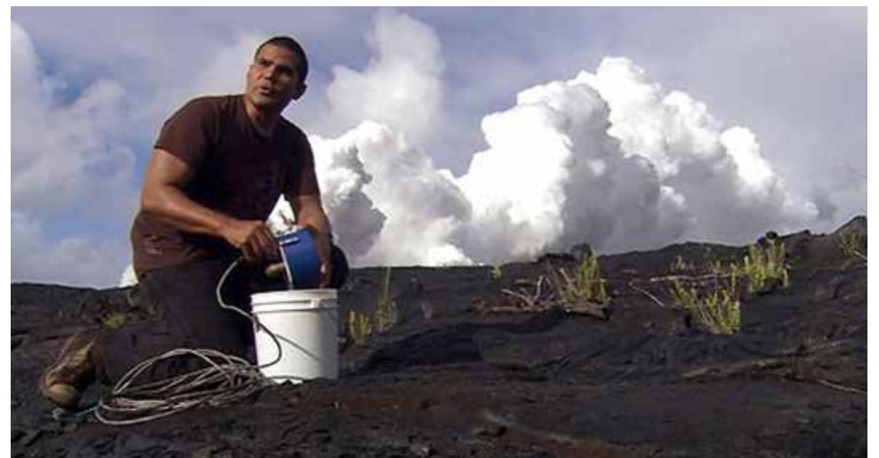
Milton Garces deploying an infrasonic microphone at Kīlauea, 2006. University of Hawai'i Infrasound Laboratory. USGS Photo
