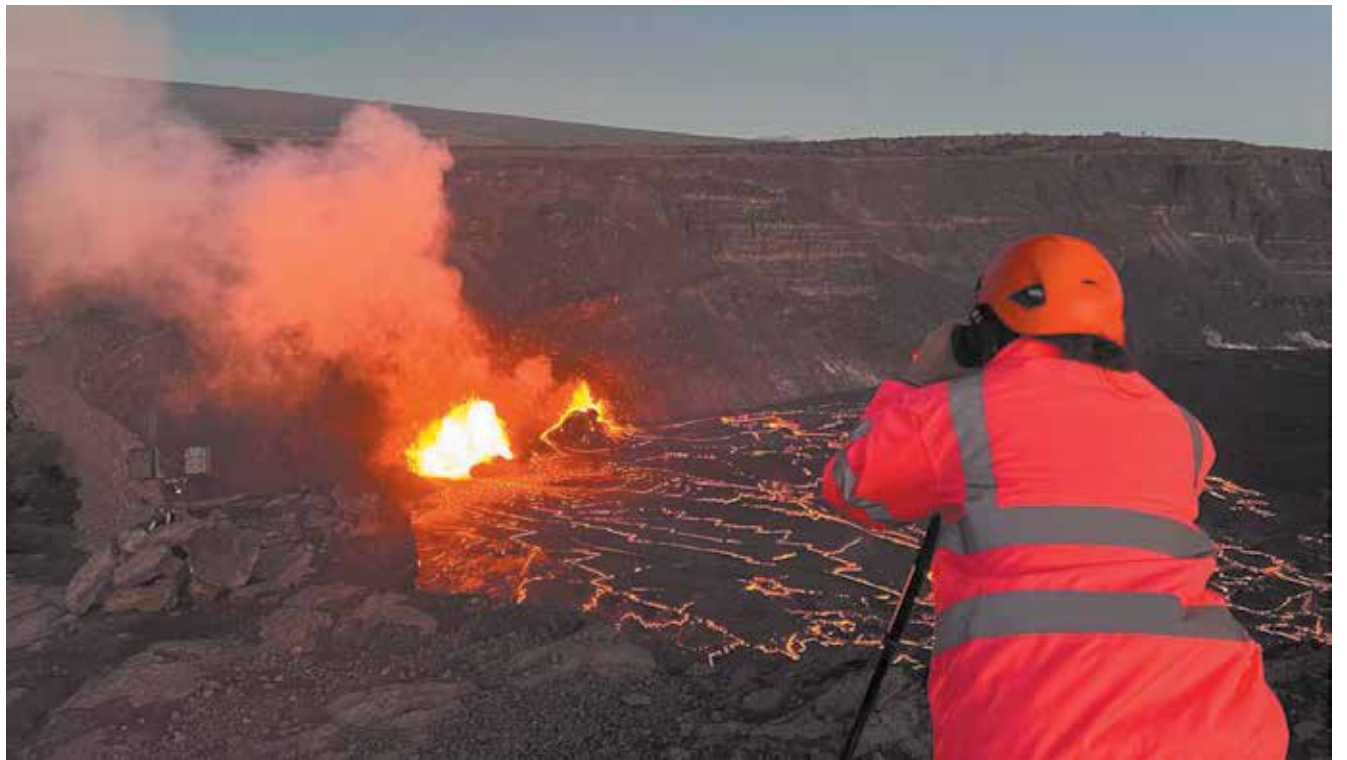
A USGS Hawaiian Volcano Observatory geologist uses a laser rangefinder to collect fountain height measurements from the eruption within Halema'uma'u crater at the summit of Kīlauea volcano. Fountain heights reached approximately 30–35 m (100–115 ft) on the morning of December 30. The S 2 cam webcam on the south rim of Halema'uma'u crater, is visible in the bottom left corner of the photo. USGS photo by H. Winslow
